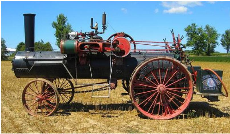
**Photo: 8 - A steam tractor, early 1900s from which power could be taken to drive other machinery, like threshers.**
